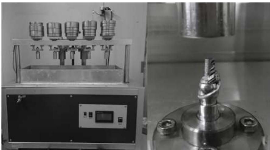
Fig. 2. Testing apparatus provided a repeated insertion/removal motion (crosshead speed: 950mm/min) up to 10,000 cycles in distilled water at 37°C, to simulate the placement and removal of RPDs.
